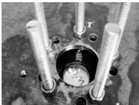
Figure 12: The magnet positioning piece was not correctly positioned on the second rotor disk, so new holes had to be drilled for the bearing mounting studs.
