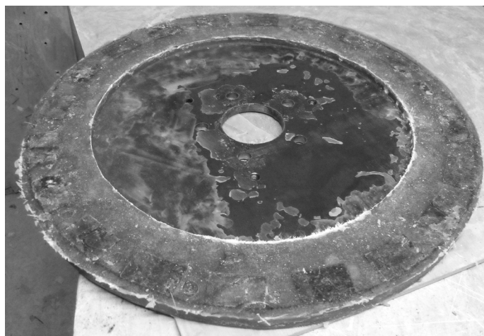
Figure 5: The generator's rotor as it came out of the mould: Neodymium magnets cast in polyester resin.
