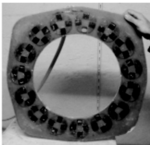
Figure 6: The generator's stator: Coils cast in polyester resin.
