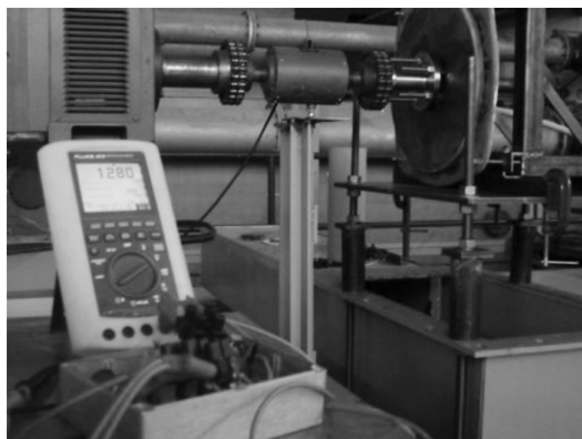
Figure 14: Testing the generator in the laboratory with the use of a variable speed DC motor drive.
