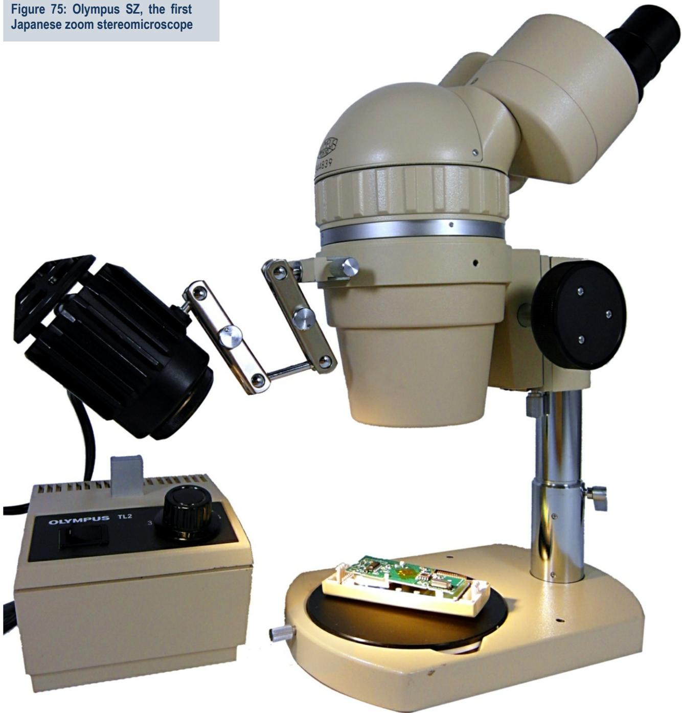
The microscope shown here is an early version, later versions are finished in "ripple pearl". The SZ microscope had an almost 30-year life, being replaced, by Olympus, only in 1989. This microscope has a reasonable field of view of approximately 12mm. The zoom function provided parfocal images; i.e., refocusing is not required when changing magnifications. The zoom
