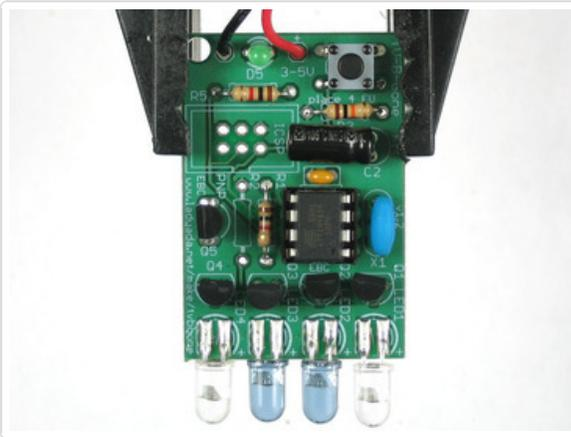
If you're in the EU, UK, Australia, place the remaining 10K resistor into **R3**. This will tell the microcontroller to use the EU database.
