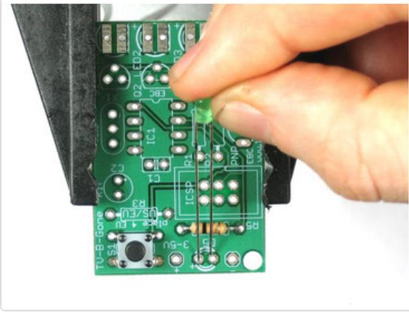
Now it's time to place the small indicator LED **LED5**. LED's are not symmetric and must be placed correctly in order to work. You'll notice one leg of the LED is longer than the other. This is the *positive* leg. The positive leg goes into the hole with a + next to it. In the picture shown, its the left hole.
