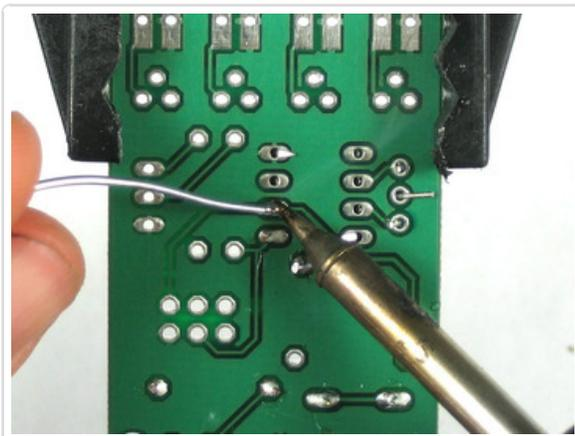
You may need to solder one pin of the socket while holding it in with a finger (or tape) as the legs aren't long enough to be bent while in place.
