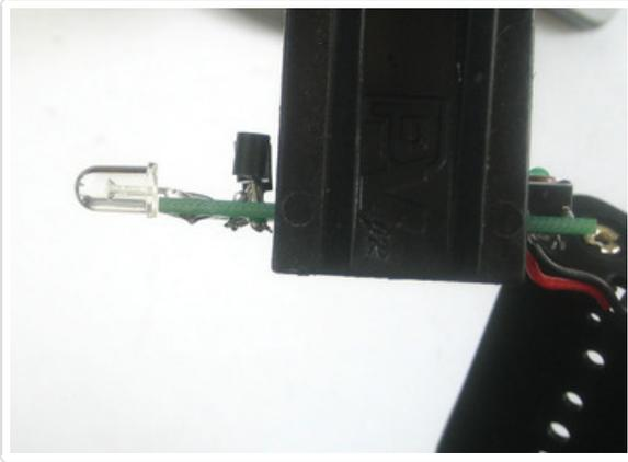
Bend the LED over 90 degrees so it sticks out over the edge of the circuit board.
