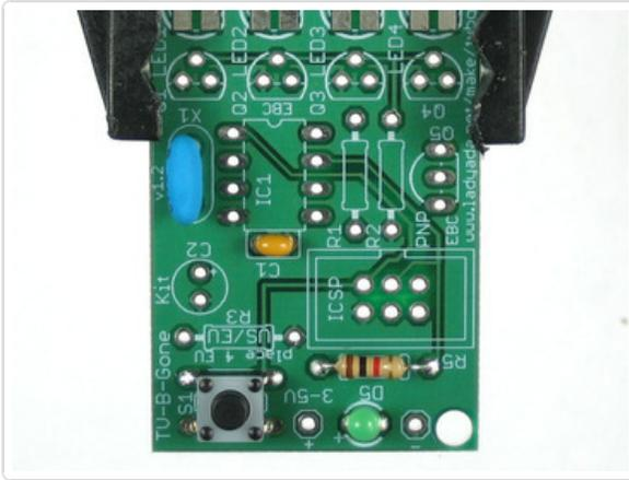
Next, place 2 components. The ceramic oscillator and the 8-pin socket. The oscillator has 3 pins and is symmetric. The oscillator is the timeclock for the microcontroller, making sure that it is performing its functions at the correct speed.
