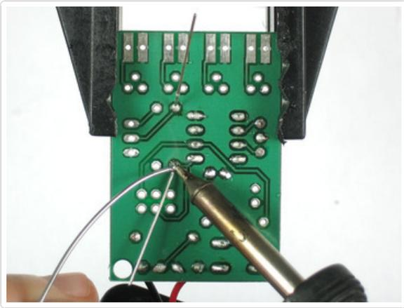
Solder and clip the resistor.
