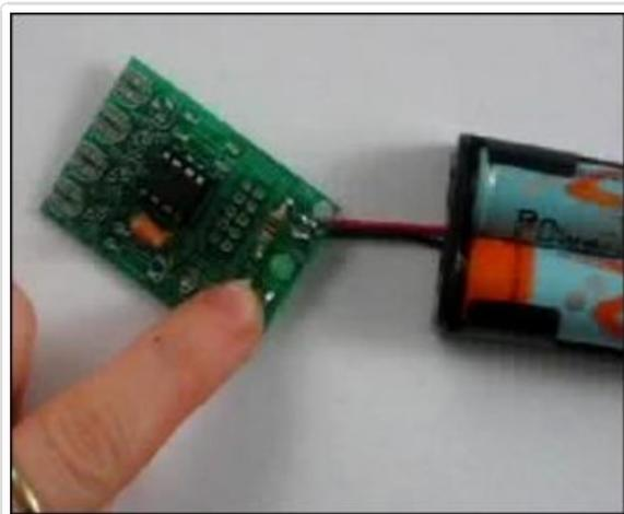
Test the kit now by putting two good AA batteries into the holder. The green indicator light should blink to show that the microcontroller is functioning properly. If you don't get a blinking light check the batteries, make sure the indicator LED is in correctly, and that the chip is in the right way.
