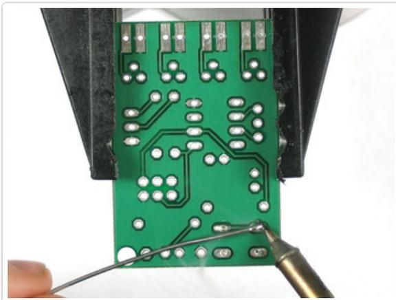
Using your soldering iron, heat up a leg of the button and the poke solder into it to make a nice solder joint.
