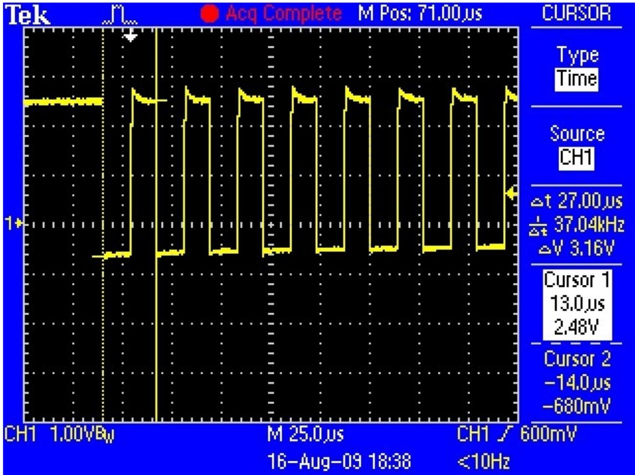
You can measure the frequency of the IR pulses. As you can tell by the cursors and the measurements on the side, the frequency is about 37.04KHz
