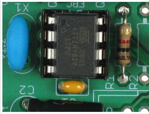
Carefully insert the microcontroller into the socket. Make sure that the little dot (and triangle) are at the end with the notch in the socket. In this photo, the dot is on the upper left.
