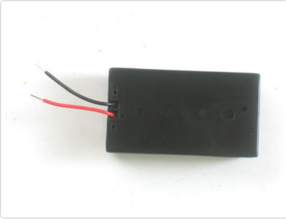
Strip the ends of the wire off so that there's a short section without insulation.
