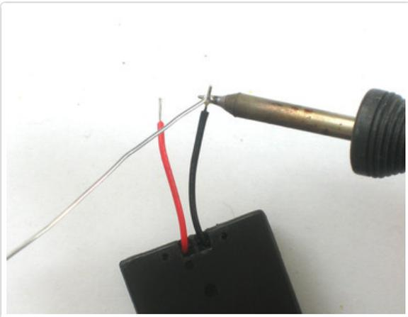
Use your soldering iron to 'tin' the wire, melting solder into it to keep the wire from fraying.
