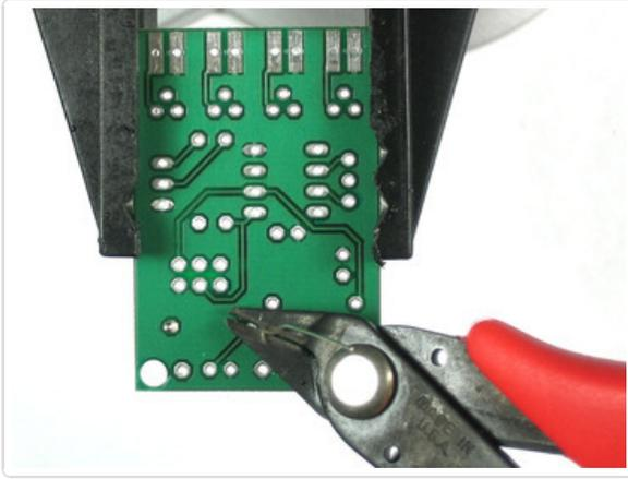
Use the diagonal cutters to clip off the resistor legs so that only the solder points remain.
