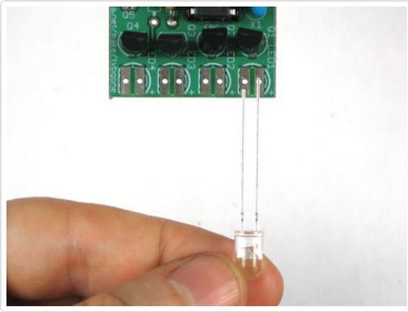
Next is the IR LEDs. Start with **LED1**, a clear IR led. Like the small indicator LED, it has polarity. Make sure the longer, positive lead is on the right, as shown.
