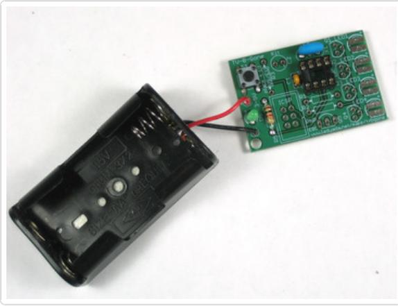
Insert the wires into the PCB so that the red wire goes to the + hole and the black wire goes to the - hole.
