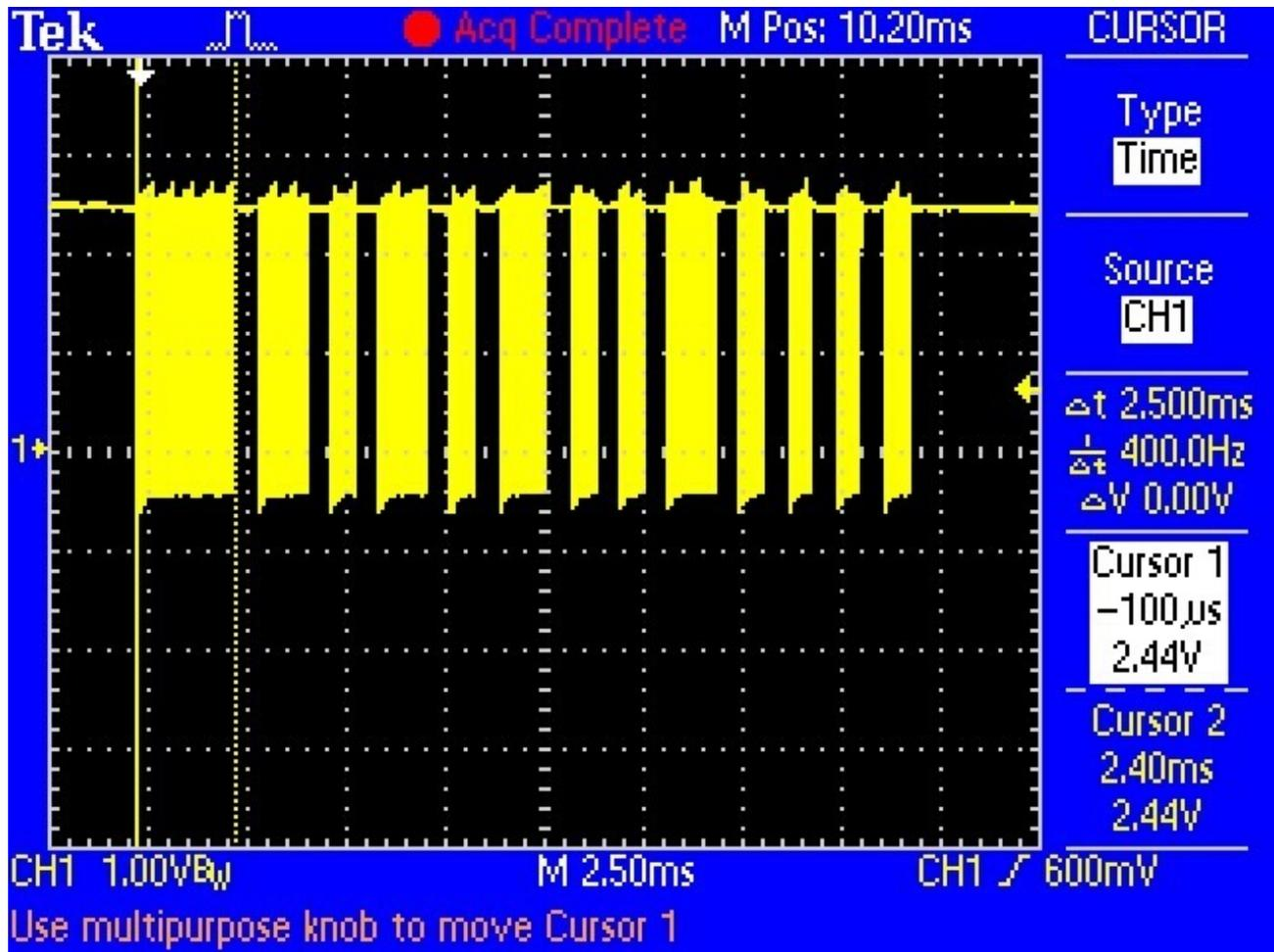
The first pulse is 2.5ms. We can use the cursors to measure the remaining pulses. I'll spare you the 12 images and let you know that the pulses are:
