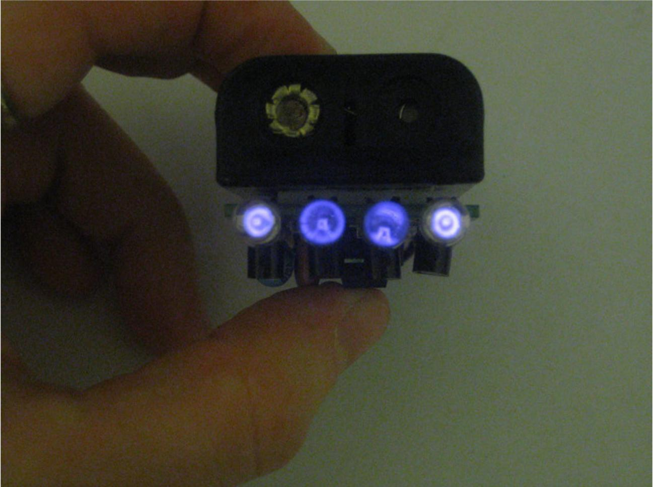
Digital cameras can detect infra-red light but our eyes can't. Use a digital camera, webcam or camcorder and look through the digital viewfinder at the IR LEDs, after pressing the button, the LEDs should flash.
