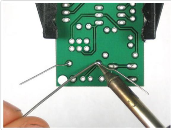
Solder each leg of the resistor.
