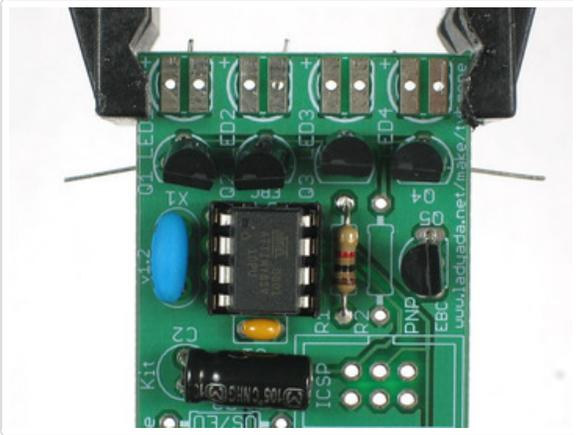
Next are the four NPN (2N2222) transistors **Q1 Q2 Q3** and **Q4**. These are the devices that turn on and off the high power IR LEDs. The microcontroller doesn't have the capability to provide a lot of power directly to the LEDs so these transistors assist it.
