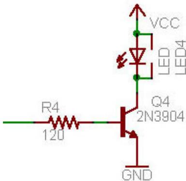
The IR LEDs have more than 100mA going through them. This is way more than a microcontroller pin can supply (usually 20 to 40 mA max!) so we use a 'driving' transistor. These NPN transistors amplify the power of a microcontroller pin and are designed to turn off currents of over 100mA. When the base pin is pulled high (through the base resistor) the transistor turns on and the LED turns on too. When the base pin is pulled to ground, the transistor turns off and no current passes through the LED.
