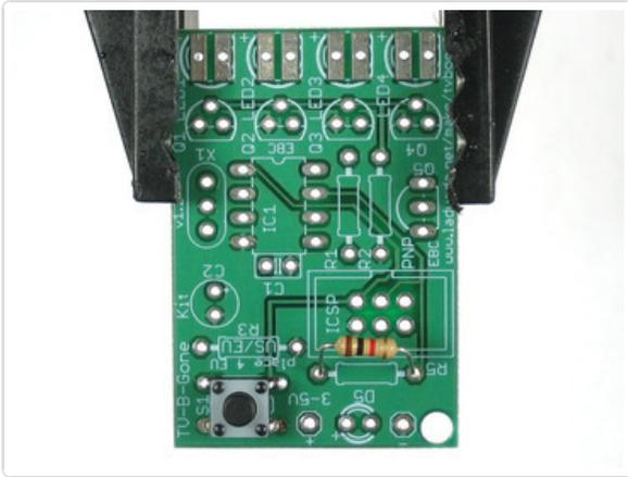
Next is the 1.0 kilo ohm resistor **R5**. This is the brown-black-red striped part. This resistor sets the brightness of the little indicator LED. Resistors are symmetric, so it can go in either way.
