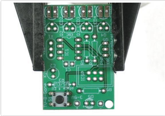
The first part we're going to assemble is the button. The button is a symmetric part so it can go in two ways. Line up the metal legs with the holes in the circuit board and snap it in. The button should sit flat against the circuit board.
