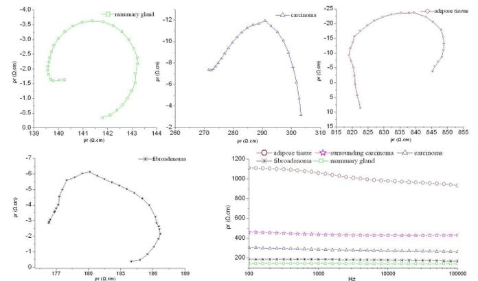
Figure 3. Impedance spectroscopy measurement for breast tissues.
