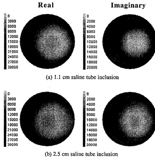
Figure 1. Reconstructed  $k^2$  images of an 8.2 cm diameter breast tissue sample with saline tube inclusions at 900 MHz: (a) 1.1 cm diameter saline tube, and (b) 2.5 cm diameter tube.
