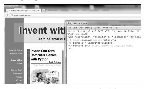
Figure 11-7: After calling webdriver.Firefox() and get() in IDLE, the Firefox browser appears.
