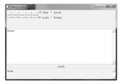
Figure 10-1: The Debug Control window
