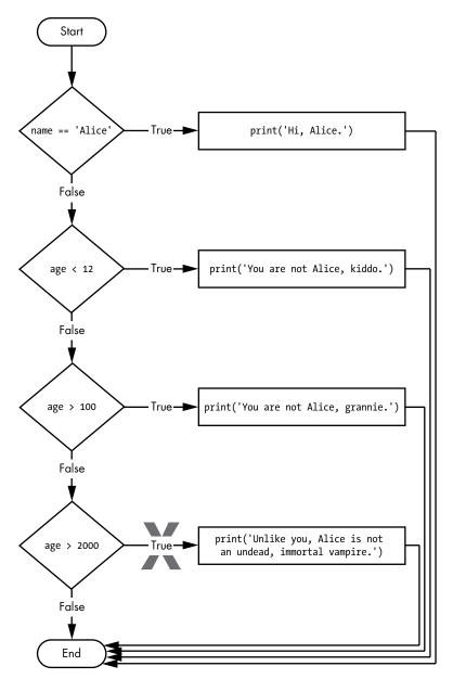
Figure 2-7: The flowchart for the vampire2.py program. The crossed-out path will logically never happen, because if age were greater than 2000, it would have already been greater than 100.
