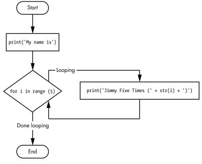
Figure 2-14: The flowchart for fiveTimes.py
