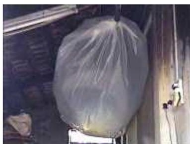
**Photo 15.** The reservoir bag full of biogas
