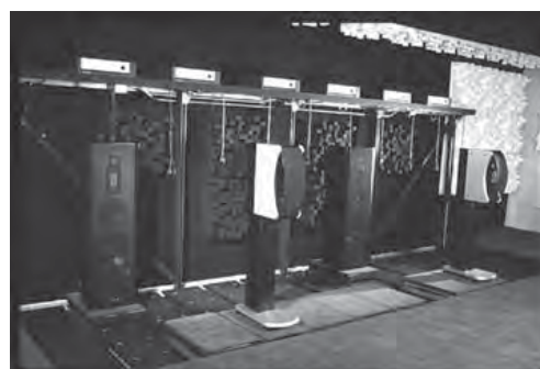
FIGURE 17.17 A photograph of a stereo loudspeaker comparison, showing two products in the forward, active locations and two others parked quietly at the wall.
