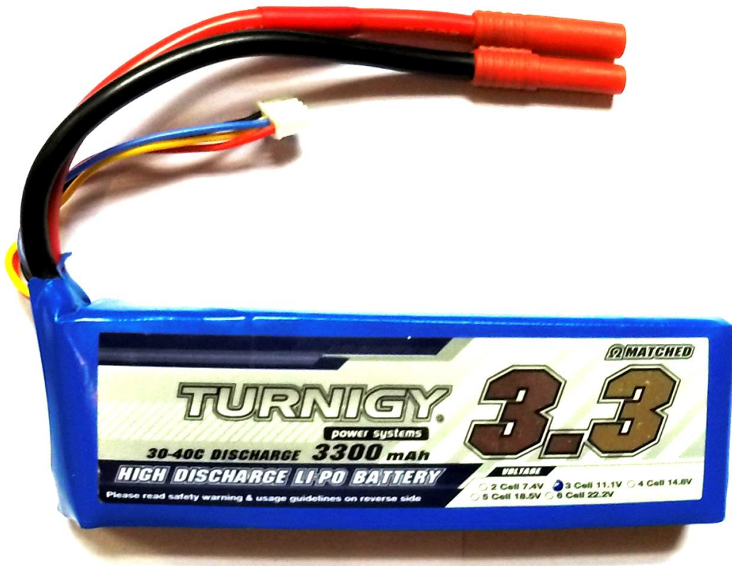
Figura 17: Bateria Turnigy Blue – 3300mAh, 3S, 30-40C.
