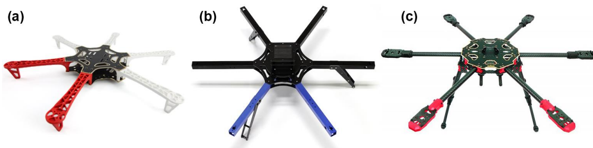
Figura 9: Estruturas comerciais de Drones: Dji Flamewheel x550, 3DR Hexa-B, Tarot 680PRO (DJI, 3DR, Hobbyking, 2015).
