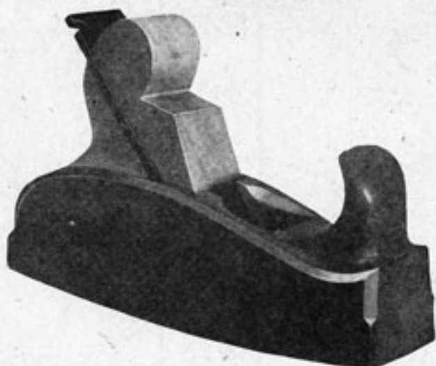
FIG. 1. MADE IN BOX OR SIMILAR HARDWOOD The length of the plane is 4\frac{1}{2} in. though a little more or less would not make much difference. The mouth should be kept small.
