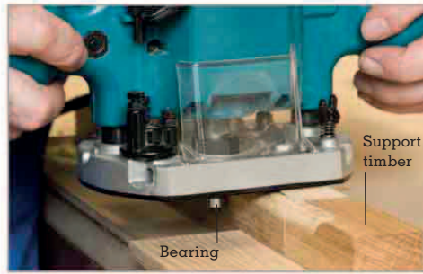
CUTTING A PROFILE WITH A BEARING-GUIDED CUTTER
