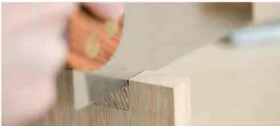
Cutting accurately to the waste side ensures precision.
