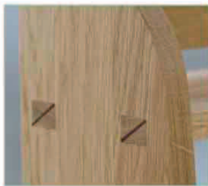
WEDGED TENON DETAIL
