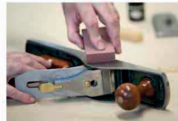
CLEANING WITH AN ABRASIVE BLOCK
