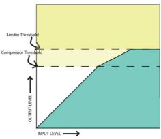
weaker signals. The limiter compressor acts as an automatic volume control and will make sure the transmitted sound is as loud as it can be, but not over modulated.
