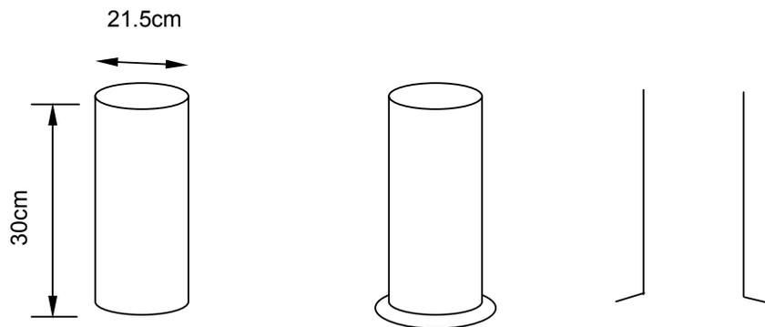
Use the hammer and anvil to spread out the shape of the base. This forms the chimney base.
