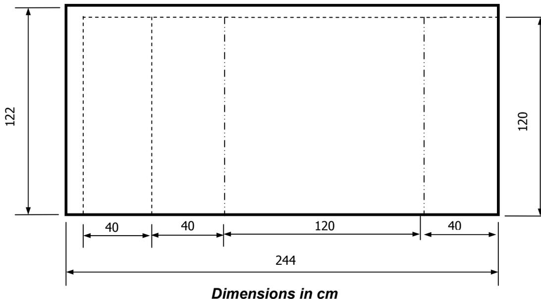
Diagram 6: Partitioning of the 4mm metal sheet to form metal box (Baking chamber)
