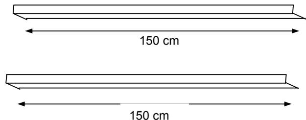
Using arc weld, attach the angle sections to the top covers as shown in figure 32 in order to align the covers and seal the joints to minimise heat escape during the time of oven operation in future.
