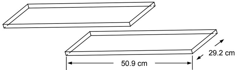
6.16 With the edges at an angle of 45°, cut the hollow section (sq. 25 X 6000 X 2 mm) into segments of the lengths specified below. These will be used to make the 2 door frames.
