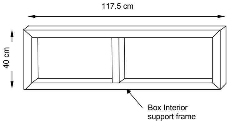
6.7 Weld two hollow section segments of length 117.5 cm on the M.S. plate assembly, as shown, to increase its structural strength. The spacing between them should be approximately 57.5 cm. (Also refer to the metal box drawing in diagram 5). Position them starting from the back while leaving a 2.5 cm gap towards the front of the box to accommodate the oven door frame to be fitted later.
