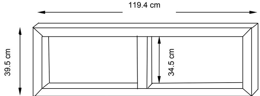
Weld the rectangular doorframe to the entrance of the metal box as shown in figure 27.
