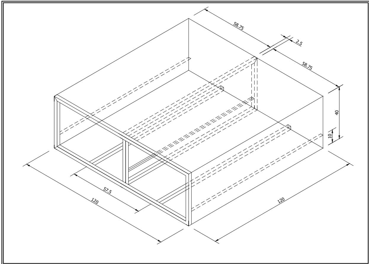
Diagram 5: Illustration of the metal oven box for the single deck oven (120 x 120 x 40cm)
