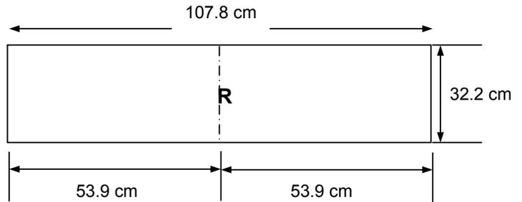
Cut out 1.5 cm squares from the corners of each of the two metal sheets cut from **R**.
