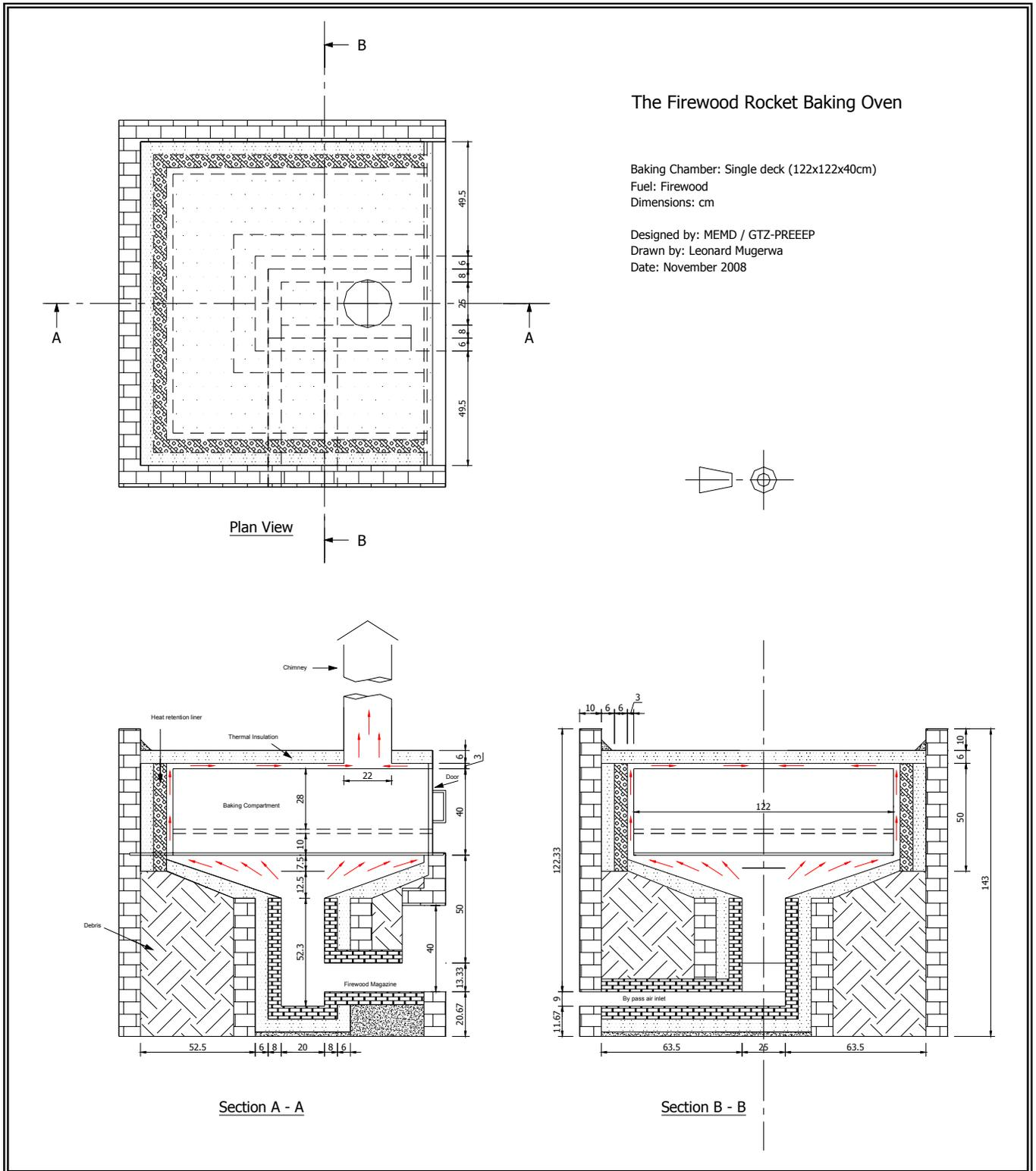
Diagram 2: Technical Drawing of the single deck Rocket Firewood baking oven
