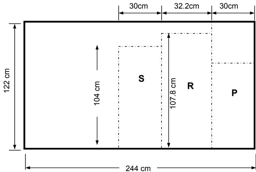
6.15 Cut out segment **R** and divide it into 2 pieces of equal length each of 53.9cm.
