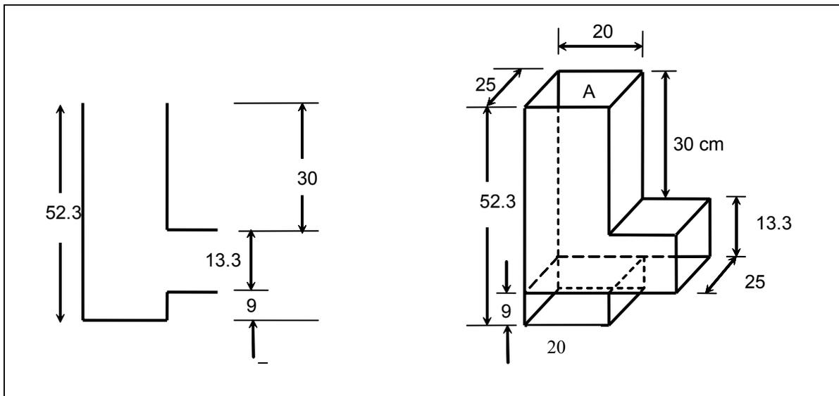
Diagram 4: Details of the combustion chamber size (Dimensions in centimeters).
