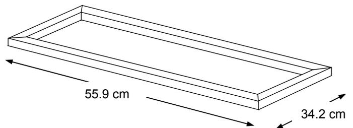
6.18 Use arc weld to fit the tray – shaped pieces into the door shutter frames. They will then appear like a tray bounded by a hollow section frame. (Figure 28)
