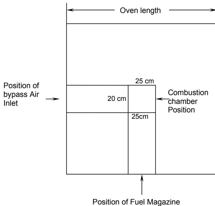
**Diagram 3: Positioning the fuel magazine and Bypass air inlet**
