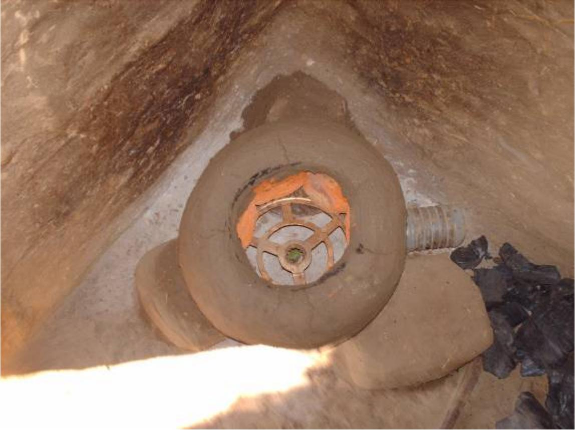
Here is a top view showing the sprocket sitting on three stones with six insulated half bricks on top of the sprocket. I'm not sure what the tin can on the right is doing, if anything. Air can enter from the bottom on all sides. Charcoal is seen waiting to the right. If you can't buy a sprocket, you can improvise with metal bars, rods, or wire, etc.
