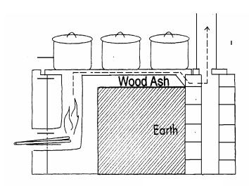
The type of material (cement brick, adobe or metal)) that is used for the exterior stove body will not have a great impact on the performance of the stove. Special materials are not needed for the stove body. The stove will function effectively as long as the body of the stove can support 5 pots and can withstand temperatures of up to 500 degrees Fahrenheit.
