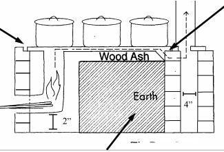
The insulation should begin to slope down 3 inches before it reaches the interior wall. This creates a passage that allows the hot flue gases to exit to the chimney.
