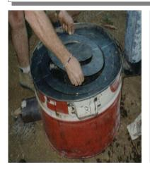
With the rings in place, multiple pots or tortillas can be cooked at the same time. The rings can also be removed for use with individual round bottom pots.
