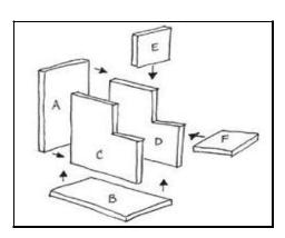
Then connect the pieces as shown. Use a 50% sand/50% clay mortar to connect the pieces. Once in use, the weight of the insulation will keep the elbow in place but it should be checked periodically to assure that it is still properly connected.
