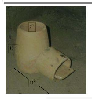
The combustion chamber can be made from refractory cement, refractory ceramic, 1/8th" steel, or cast iron. We are also experimenting with a ceramic tile (see page 7) from Guatemala and our own refractory mix.
