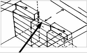
KEEP THIS SPACE UNOBSTRUCTED. DO NOT FILL IN THE GAP OF THE INTERIOR WALL'S LAST BRICK LEVEL
